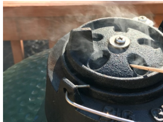
Figure 2. The correct opening, 1/16" wide (top picture), just enough for inserting the tip of a toothpick (bottom picture). This configuration applies to all kamado styled smokers. Smokers with single layer sheet metal such as the Weber Smokey Mountain needs 1/4" or wider opening on the top vent.
