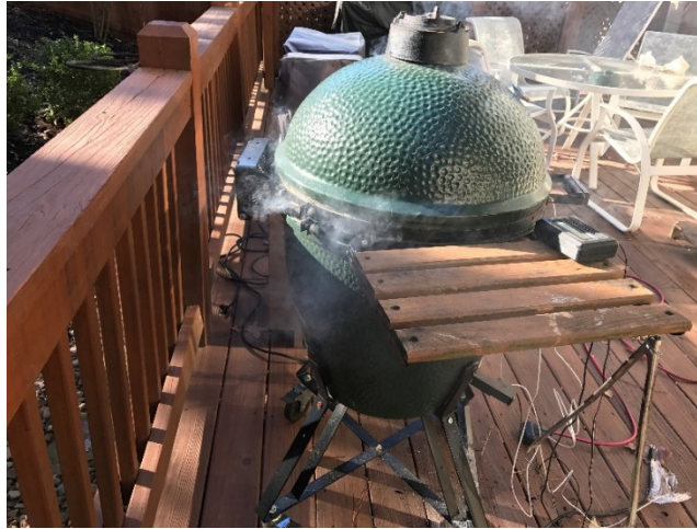
Figure 3. Air or smoke can leak from the gap between the dome and the smoker. Poor air seal can lead to poor temperature control.
