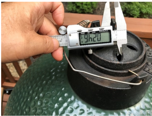
Figure 1. In the picture on the top, the opening of the top vent is 1/4" wide, which is too large for an 18.5" Big Green Egg smoker cooking at 225°F with ambient at 40°F. On the temperature chart on the bottom, the pit temperature stays above the set temperature even when the fan has stopped running from 14:47 to 15:40. This problem is corrected by closing down the top vent to 1/16" wide.
