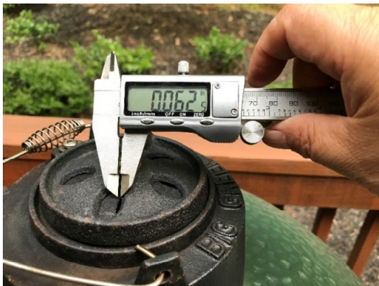
Figure 2. The correct opening, 1/16" wide (top picture), just enough for inserting the tip of a toothpick (bottom picture). This configuration applies to all kamado styled smokers. Smokers with single layer sheet metal such as the Weber Smokey Mountain needs 1/4" or wider opening on the top vent.
